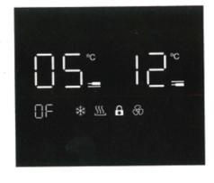
The display window can be set to the off position for a less obtrusive appearance. Your Wine Cooler will continue to run, but the Wine Coolers display window will not be visible. You can check the temperature of the Wine Cooler by pressing the **Power** button.
